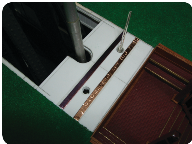
Photo 312. The circuitry for the LEDs that will illuminate the opposite end of the engine room.
