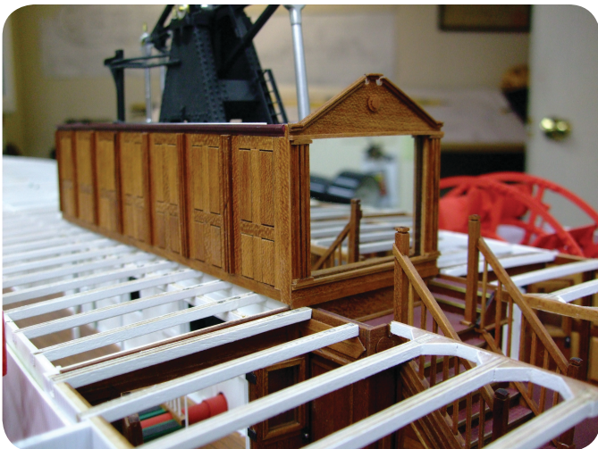
Photo 307. The enclosure in place at the first landing of the grand staircase. A real mirror has been included.
