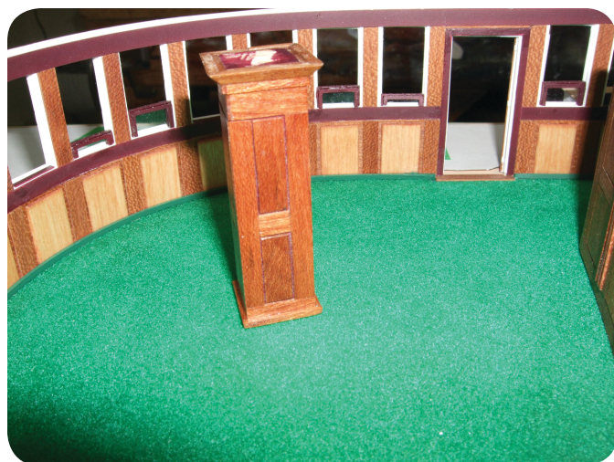
Photo 313. The third structure found on this deck served as a conduit for the gear that passed down from the wheelhouse on its way to the machinery.
