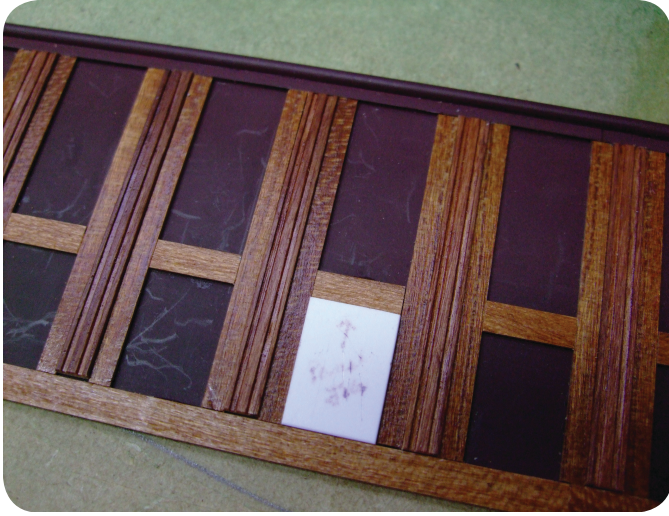
Photo 295. The white jig shown here sets the height of the horizontal Frames. Note the pillar facades that are found centrally in the frame.
