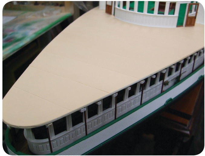
Photo 289. The deck is resting on the ceiling joists after they were marked and cut back to align with the edge of the deck.
