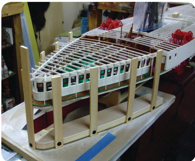
Photo 285. The support beams for the salon include the longitudinal ones, provided support for the ceiling joists.
