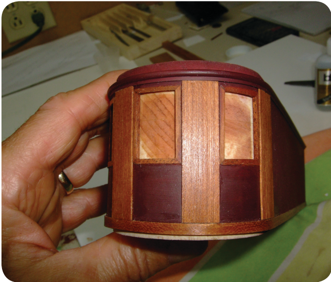
Photo 301 to 305. The steps in paneling. Note in the photo above the window frame has been added.
