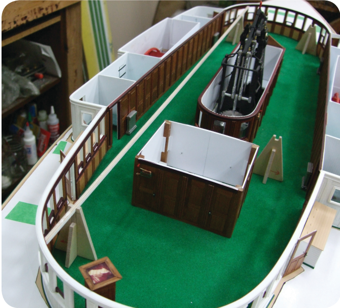
Photo 319. Determining the correct length of these beams proved difficult as they needed to be located relative to the center of the space and match the width of the turtle deck.
