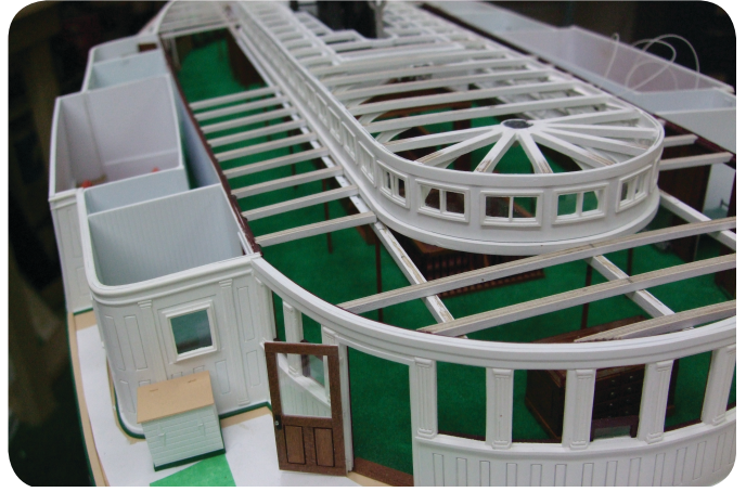
Photo 317. The unfinished turtle deck rests on the longitudinal support beams.
