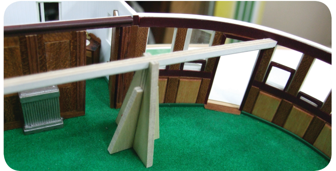
Photo 318. A closer look at the beam jig that needed to be self-standing and conform to the camber of the deck.
