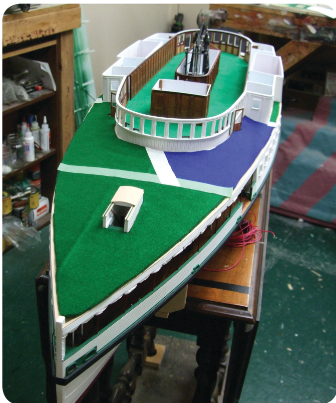
Photo 275. The finished forward companionway is surrounded by a protective layer of felt.
