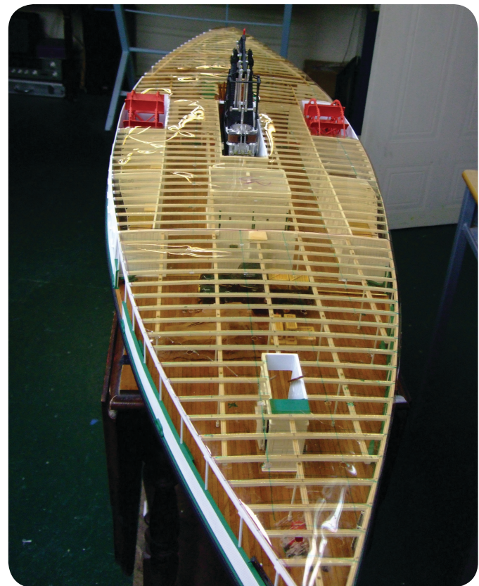
Photo 245. The first step in the process required for the installation of LEDs. The yellow jell allows the siting of the LED to be free of support structures.
