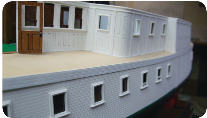
Photo 281 and 282. The covering for the deck edge consisted of tongue in groove treated with butt ends and then a composite applied over it.
