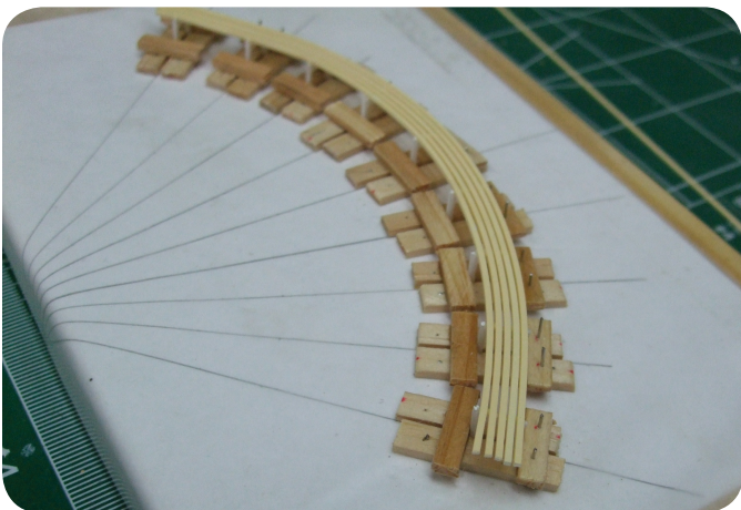
Photo 280. The bench is nearing completion while being held in the jig.
