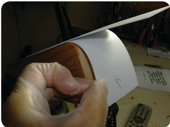
Photo 267. The jig and laminations used to build up the rounded corner for these walls.
