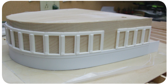
Photo 261. The jig plug for the aft rounded building and the partially finished structure.
