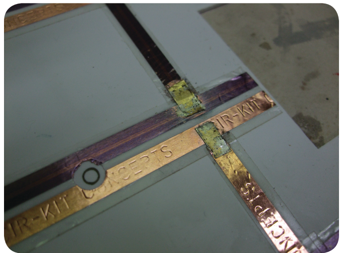
Photo 252. This is the endpoint chosen to accept the hook up of the power source into the circuit.
