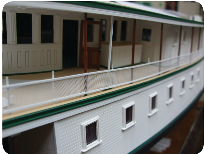
Photo 281 and 282. The covering for the deck edge consisted of tongue in groove treated with butt ends and then a composite applied over it.
