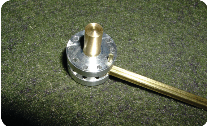
Photos 228 (above) & 229 (below). The assembly of the inside portion of the cam rod to the hub. The drive rod hasn't been fixed in position at this point.
