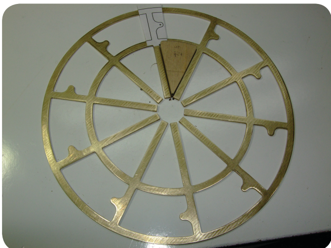
Photo 196. The finished cut from brass and one of the wooden pie shapes used for the jig.
