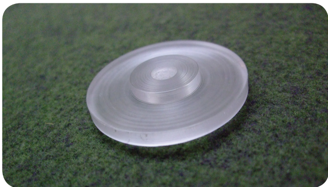
Photo 204. The finished hub. The raised center is there to accept the ends of the spokes.
