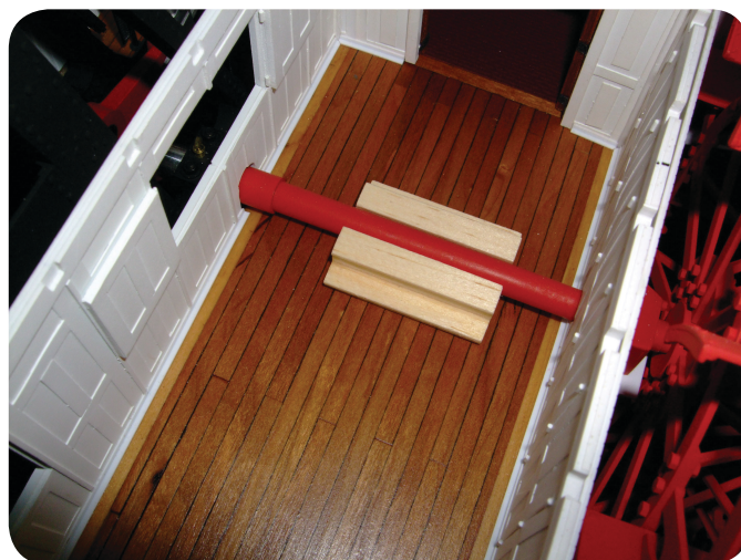
Photo 238. The main driveshaft housing passed through above the deck surface which presented an obstacle for passengers and crew. A staircase was built to solve this problem.
