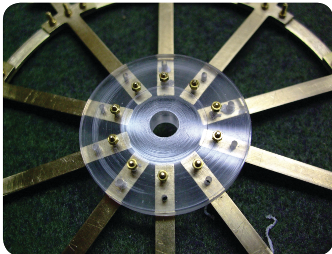
Photo 205. The outer hub has been mounted to the spokes and drilled to accept the bolt assemblies.
