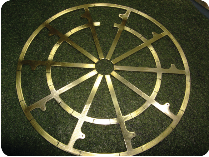
Photo 198. The first cut away of the inner ring in the process of freeing the spokes of the wheel.
