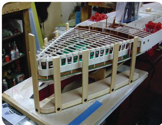
Photo 152. The form used to build up the bulwarks was used to mount pine guides that would provide support while they are glued in place.
