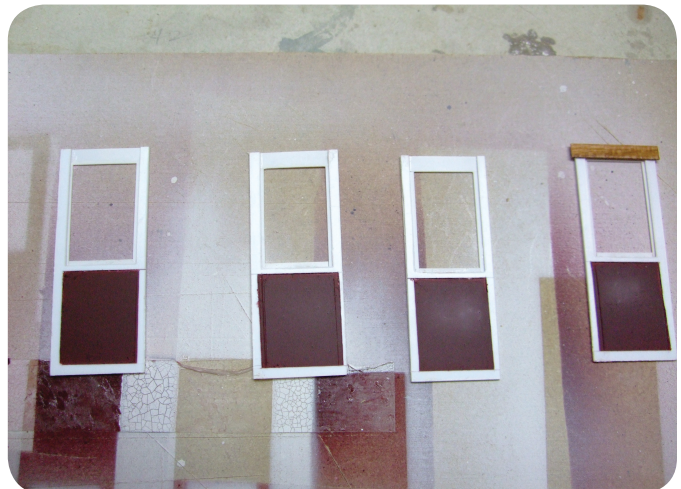
Photo 158. The core of the door has been built up to provide the pocket for the glazing. Next, the cherry strips go on. The maroon paint is used for contrast between raised panels.
