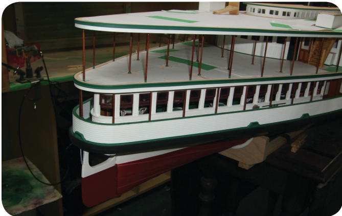
Photo 154. The bulwarks as they appear once attached.
