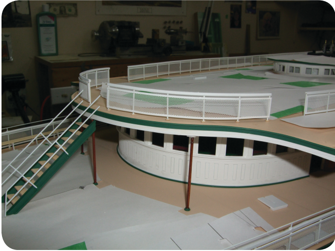
Photo 183. Each pillar needed a footing. Each of these were built on the lathe in brass and then painted green.
