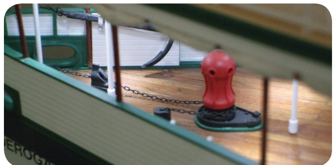
Photo 166. The chain locking ribs are shown here along with one of the two cable stoppers.
