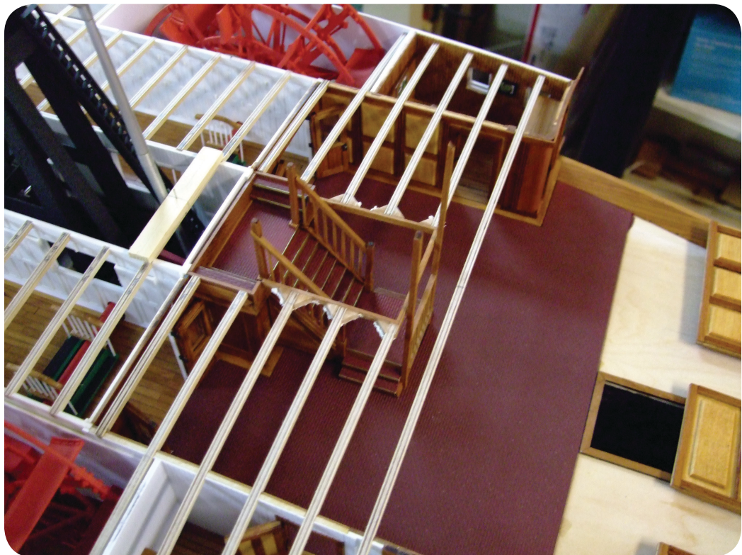
Photos 191 and 192. The ceiling beams have been installed in the central section of the first deck.
