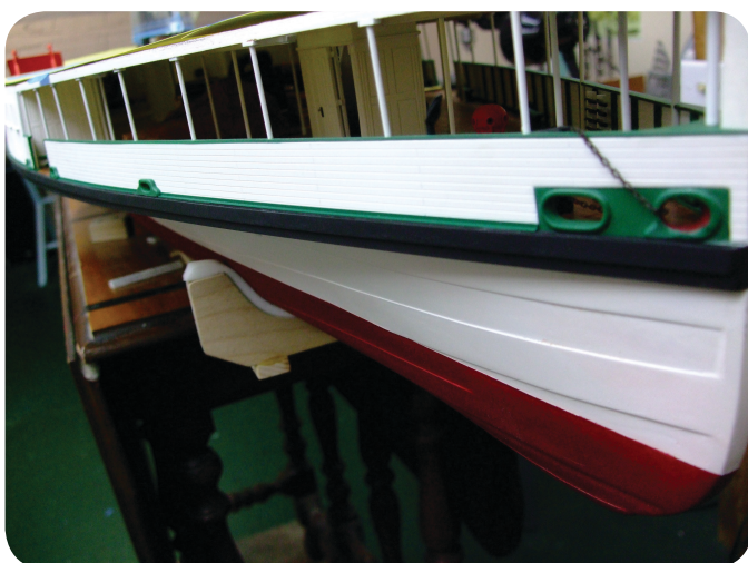
Photo 172. The finished bulwarks including the top rail and the double fair lead on both the port and starboard sides.
