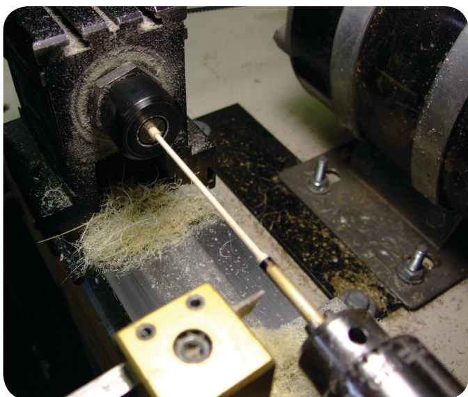
Photo 180. The configuration for the lathe for turning the bamboo pillars.
