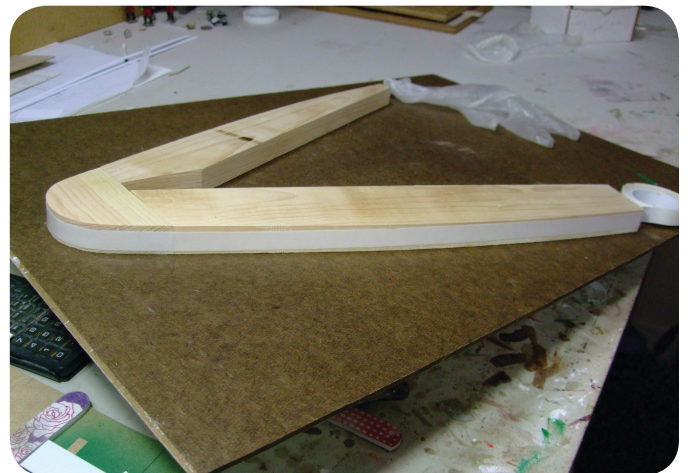
Photo 148. The jig that was used to mount the bulwarks for gluing. The two-sided tape has been partially readied for the task.
