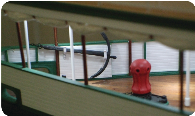
Photo 167. The anchor is mounted on the inboard side of the starboard bulwark.
