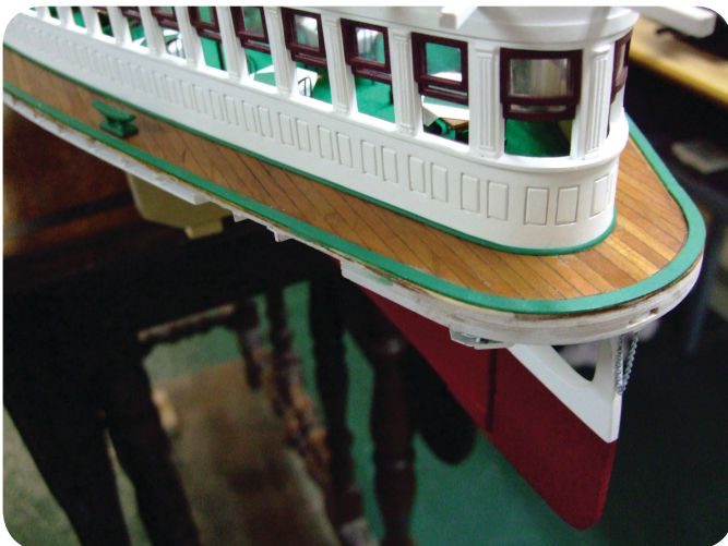
Photo 147. The walkway onto which the bulwark will be attached.
