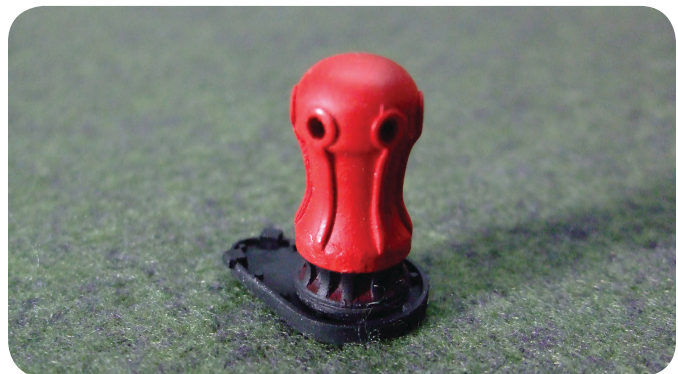
Photo 165. The capstan built up from a brass core with styrene embossed details.
