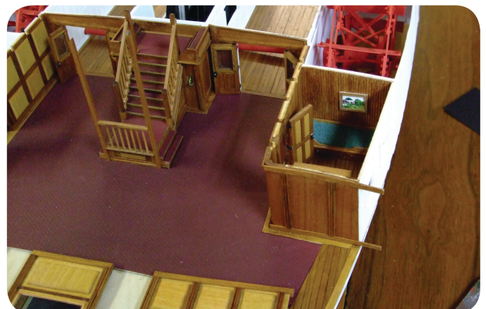
Photo 96. The area around the grand staircase was constructed in black cherry and butternut woods. The interior of the captain's quarters has been finished and will be lit by LEDs.
