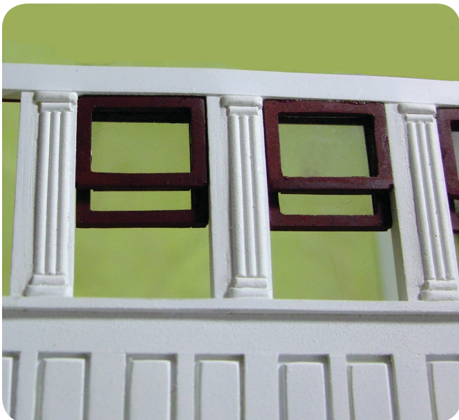
Photo 125. The quality of filling leads to an undetectable seam.
