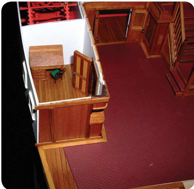
Photo 97. The interior of the Pursers office has been finished and will be lit by LEDs. Note the flooring texture in this space.
