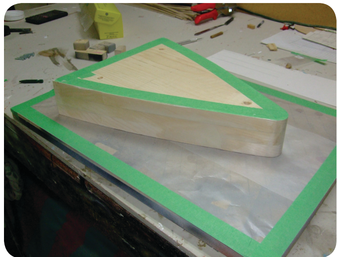
Photo 111. The plug is mounted on a waxed paper covered base. The sides were also covered.
