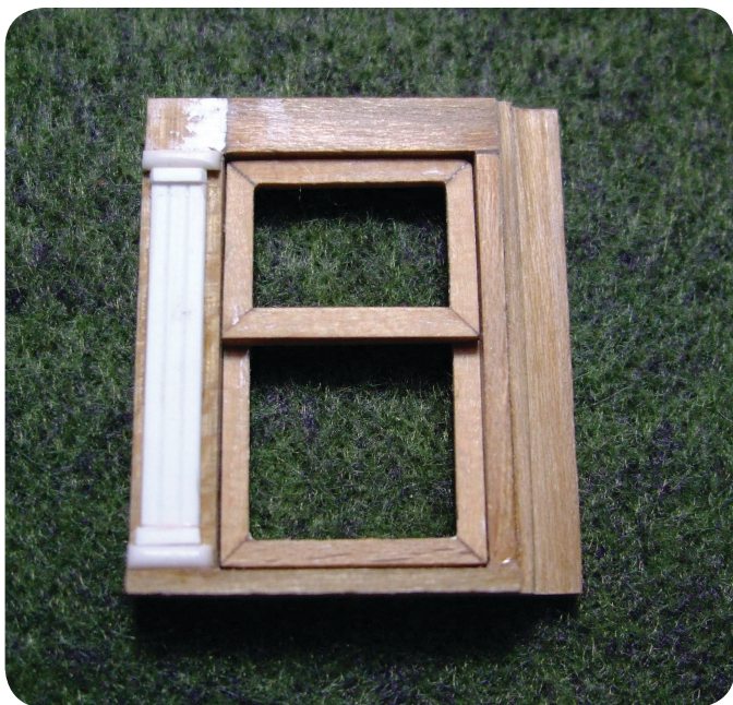
Photo 120. The master assembly for the windows.
