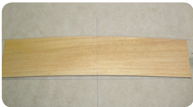
Photo 107. The one-millimeter thick core for the salon partition was cut following the contours of the deck and ceiling.
