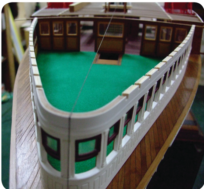
Photo 127. The header for the salon is in place ready for the beam installation.
