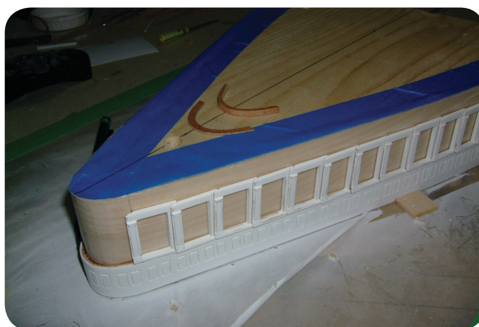
Photo 123. The window frame assembly is shown in its early configuration on the plug.
