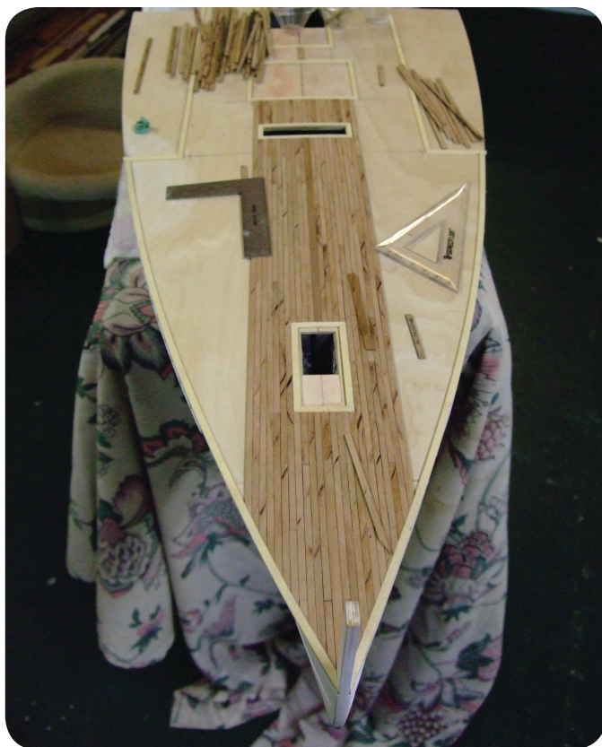
Photo 66. The “three-butt” planking has begun. Note that nibbling is not required for the planking at the water board near the bow.
