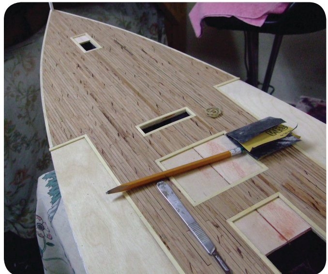
Photo 71. The forward cargo deck is ready for sanding and polyurethane application.
