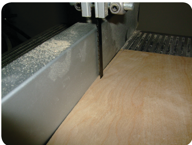
Photo 88. The fence of the band saw allowed the cut of the beam to be of a consistent depth.
