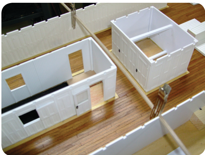
Photo 87. A ceiling beam has been temporarily installed to test for accuracy. The beam must run parallel to the adjacent wall for it to be correct and it does.
