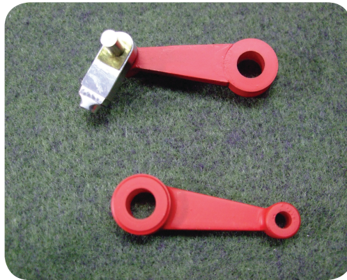
Photo 42 - 44. The two halves of the main crank built from styrene. The bearing for the main connecting rod ready for assembly. The assembly ready to be mounted in the “A” frame.
