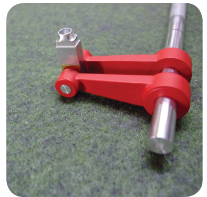
Photo 42 - 44. The two halves of the main crank built from styrene. The bearing for the main connecting rod ready for assembly. The assembly ready to be mounted in the “A” frame.
