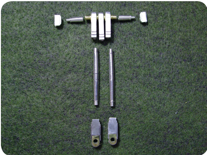
Photo 54. The metal parts required to build the crosshead assembly.
