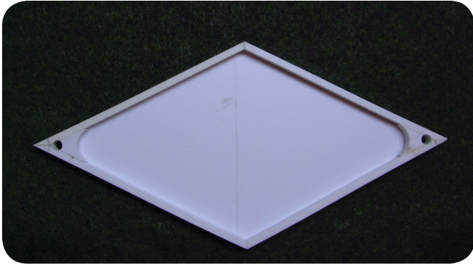
Photo 36. A thin 0.25mm sheet of styrene was glued to one side of the frame to ensure that the frame held together.
