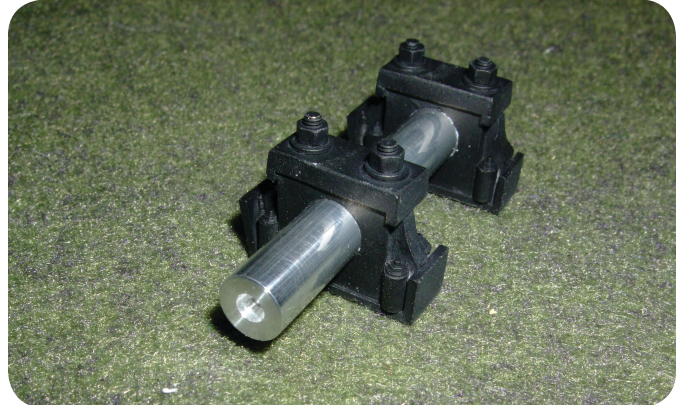
Photo 40. The two bearings for the main drive shaft and crank being tested for sizing before the brass insert was added.
