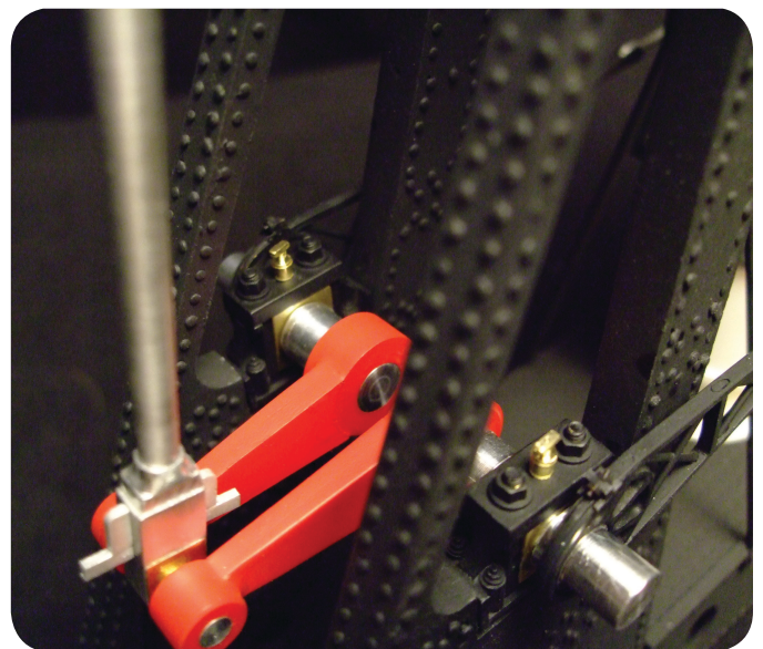
Photo 46. The connecting rod attachment to its bearing at the crank.
