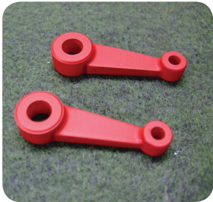
Photo 42 - 44. The two halves of the main crank built from styrene. The bearing for the main connecting rod ready for assembly. The assembly ready to be mounted in the “A” frame.
