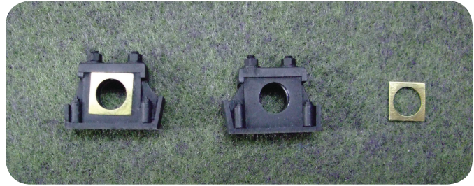
Photo 39. The painted bearings and brass insert used to simulate the brass bearing inserts.
