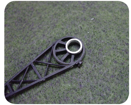
Photo 58 - 60. The eccentric bearing constructed from brass and Evergreen styrene stock with an aluminum off-center mounting ring.
