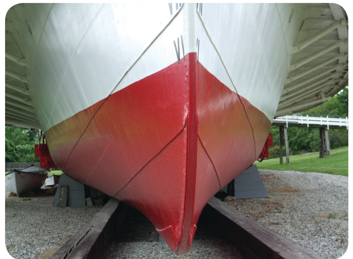
Photos 1 & 2. Notice the arrangement of the plating and the lack of rivet evidence.
