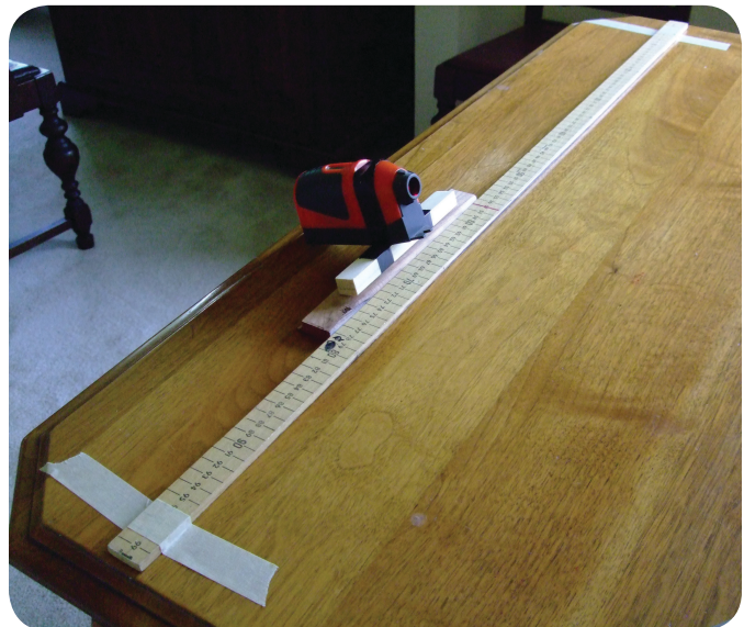
Photo 4. The laser is mounted on the block to ensure that the light wrapped itself around the hull. The meter stick guides the position of the light source.
