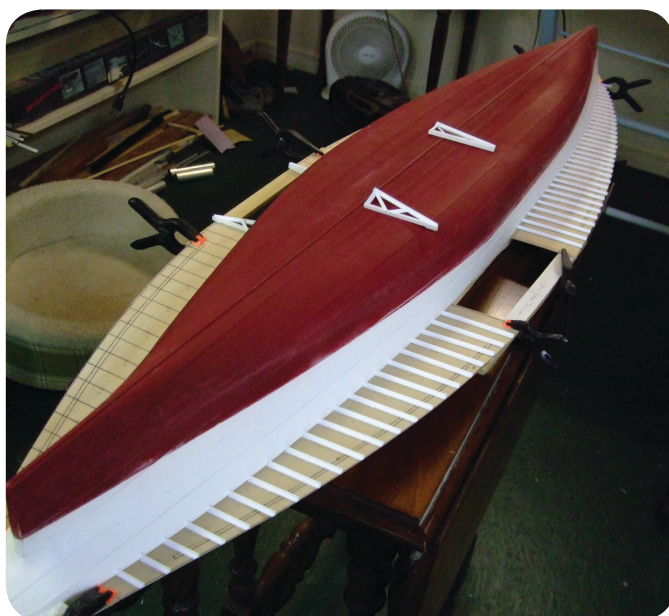
Photos 17 & 18. There were triangular support structures required forward and abaft of the paddle-wheel openings. A total of seven on each side were required.
