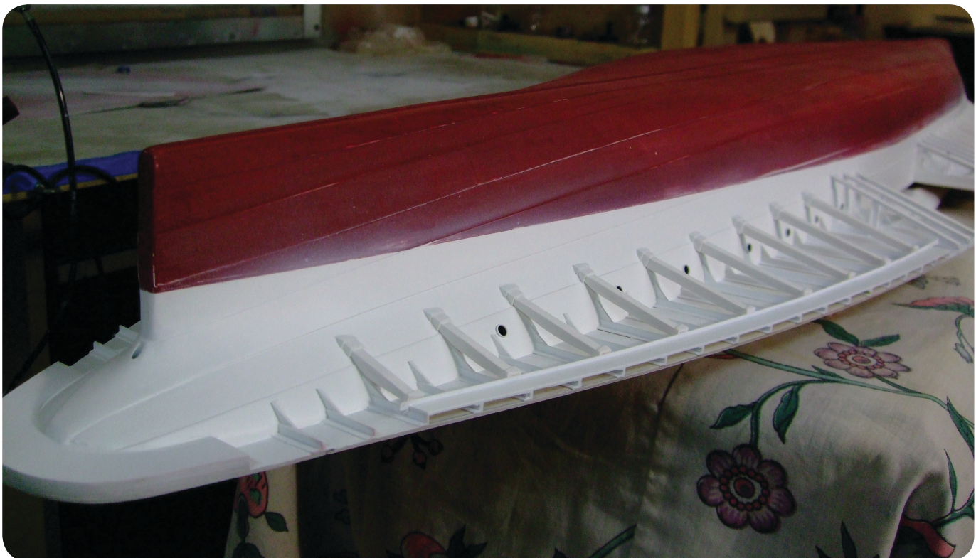
Photo 21. The portholes are in and the painted braces are mounted.
