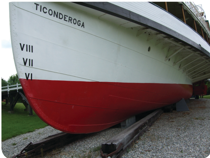
Photos 1 & 2. Notice the arrangement of the plating and the lack of rivet evidence.
