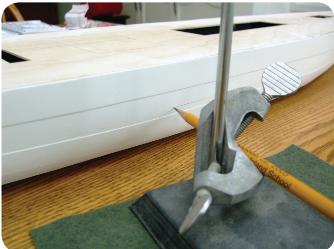
Photo 11. Marking the water line using a retort stand and clamped pencil.
