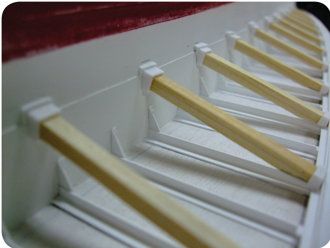
Photo 19. The next type of brace for the deck was made of wood and nesting square Evergreen tubing.
