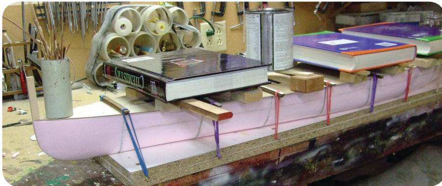
Photo 14. The 1/16" plywood deck surface is being held to ensure that a thorough attachment is achieved.
