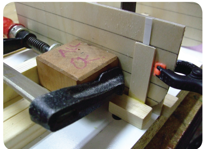
Photo 7. The apparatus used to align the body form to the keel on all three planes.
