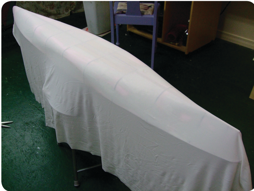
Photo 17. The ability of the cloth to drape around the stern shows its suitability for the job.
