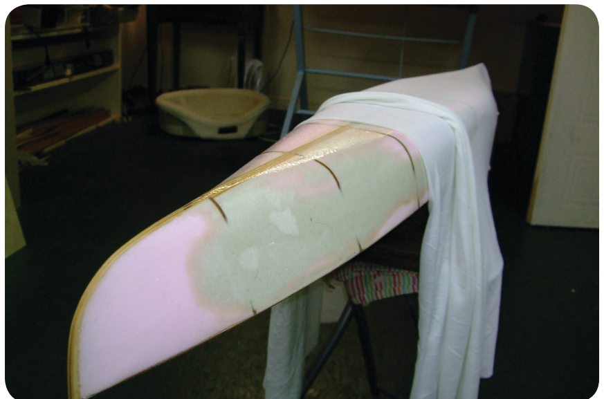
Photo 18. The hull is wetted with the epoxy before the cloth was placed onto the surface. Additional epoxy was rolled onto the cloth once smoothed over the wet hull.
