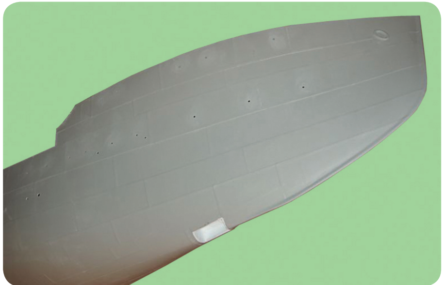
Photo 3. The forward hull showing porthole locations correctly pilot drilled and the well for the Asdic dome.
