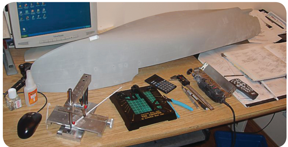
Photo 1. The Fleetscale hull, 51-1/4" long. The bulwark has been cut away, and in the foreground are the specialty tools that speeded up the work.
