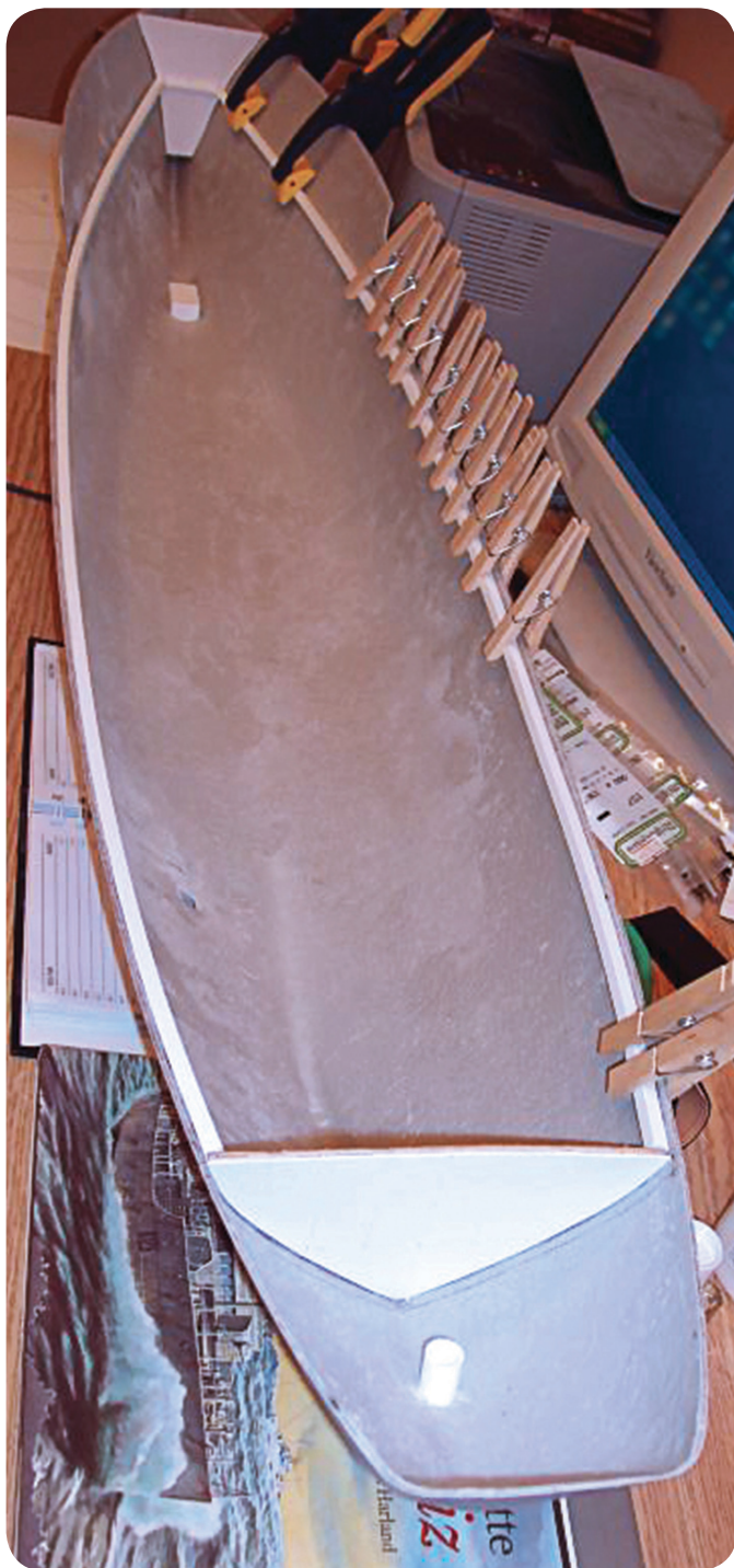
Photo 5. Main deck ledges being installed.
