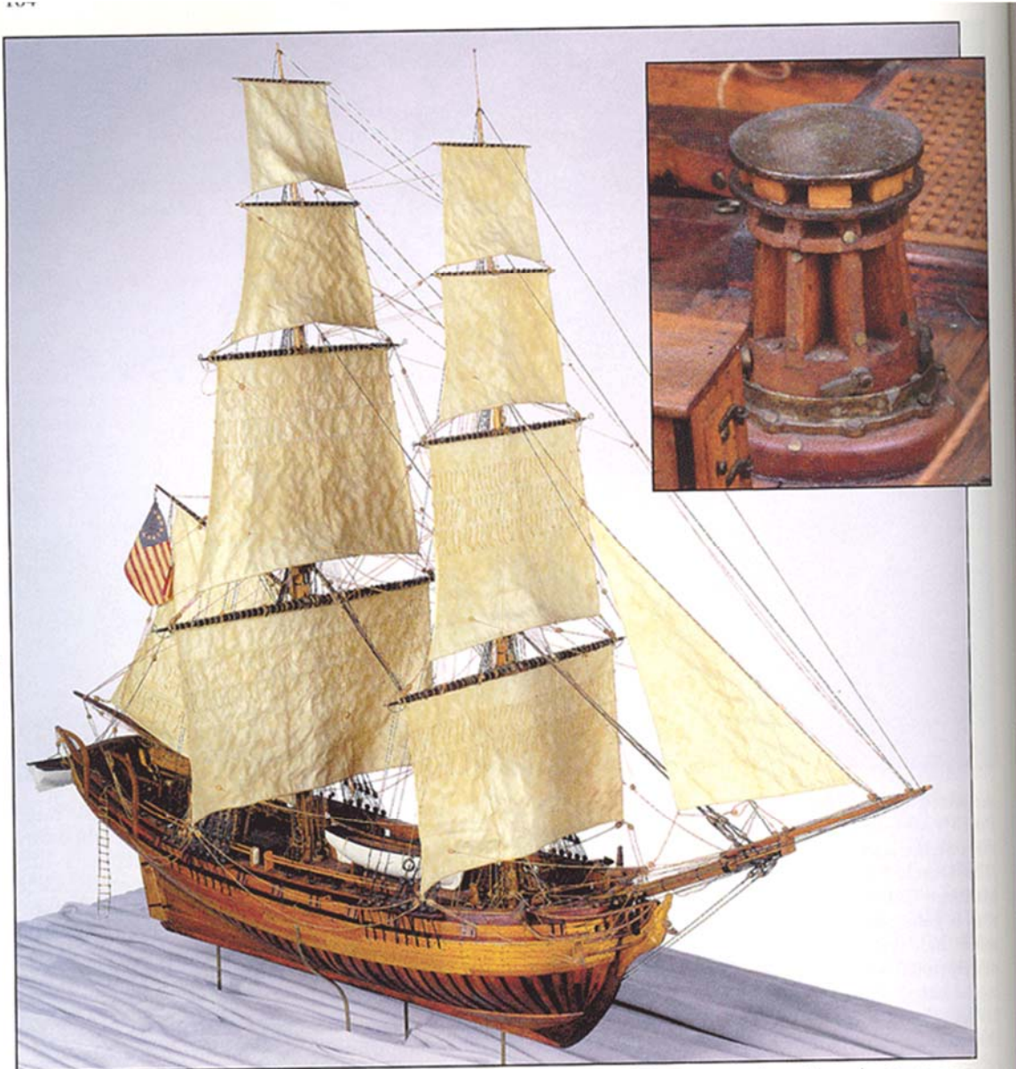
Plate 7. Armed Brig ca. 1810. In peacetime, brigs were used widely in coastal trading, short sea voyages, and training. In time of war, their speed made them useful as escorts, messengers, and commerce raiders. Brigs of war were typically about 100 feet long with a 24-foot beam, and carried 40 guns. Although Crabtree based this model on plans published in the early 1930s that were supposed to represent the American Revolutionary War vessel USS Lexington , more-recent scholarship indicates that the curved boat davits and certain details of this model's masting and rigging (such as jackstays on the yards) are more typical of brigs of the early nineteenth century. This vessel is, therefore, more appropriately dated 1810 than 1776. The sails, hand sewn by Winnifred Crabtree, are linen, as is the rigging—the most elaborate in the Crabtree collection. Length: 49 inches; scale: 3/8'' = 1' .
