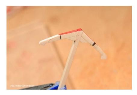
It helps to work on a sheet of thin Plexiglass, as one can use the edge as guide for the file.
