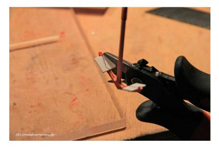
After they were glued in place, the outer edges were cut to shape. All that was left was to clean up any tool marks and paint.
