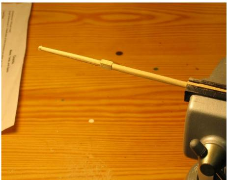
I chuck the mast into my trusty hand drill and, using a strip of 220 grit sandpaper, get a fine, smooth finish on the mast. If I happen to break the mast at this point, it conveniently falls directly into the trash can.
