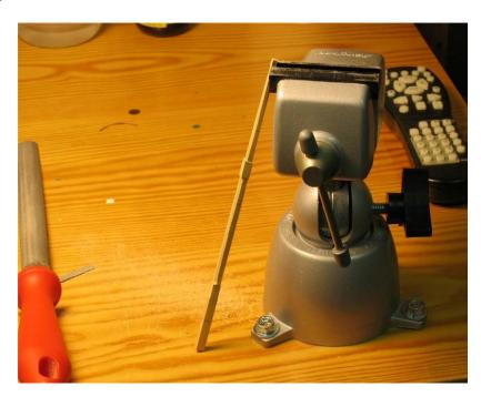
I now move on to using a fine, flat file. The next step is to turn that eight-sided mast into a 16-sided mast. Since marking the lines would cause more errors for me than it's worth, I simply filed the edges of the eight sides. With little effort the mast becomes very close to a tapered circular section. This amazes me each time I do it. It is surprisingly easy.
