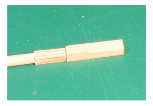
In this photo I've already filed the octagonal section near the heel and am working on the hounds. I first file the hounds to octagonal, but without the taper, and then come back and gently file the taper, working from the lower end up. This is the one portion of my process that takes some finesse.
