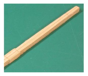
Back to the Dremel to sand the taper into the second sides of the mast, perpendicular to the first marked and sanded sides.
