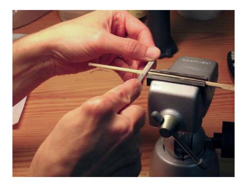
I clean up the upper edge of the hounds with a chisel; the fine flat file works well for this, too.
