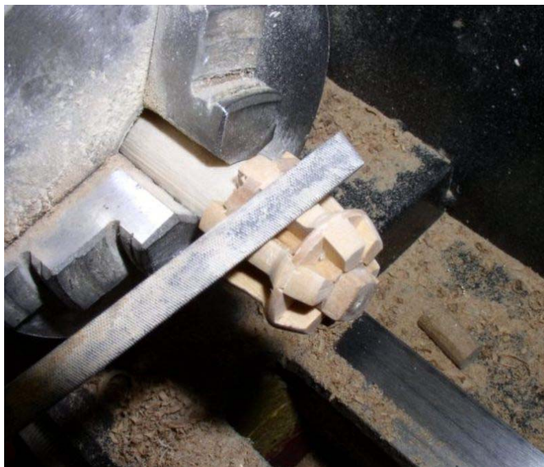
Filing the upper capstan. Note the TEMPORARY dowel that is chucked in the lathe
