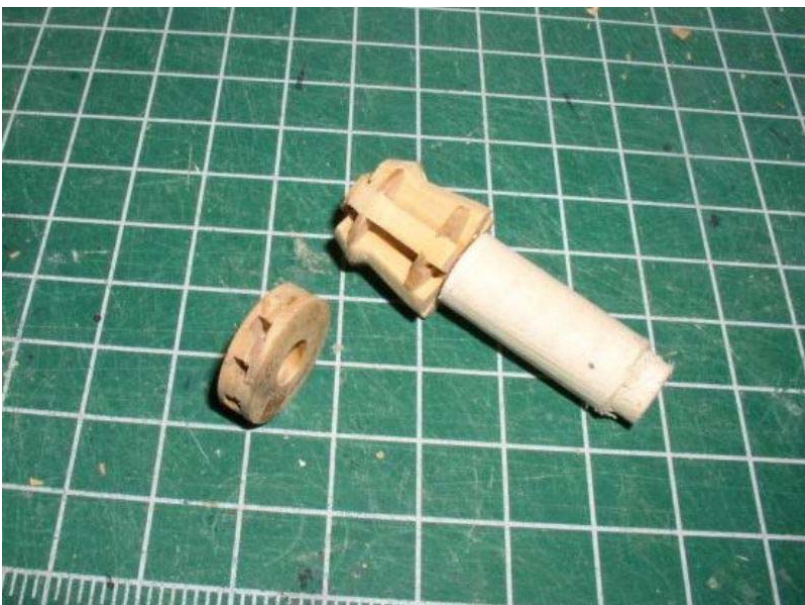
Upper capstan head and body with temporary dowel inserted. Note the hole in the center of the drumhead
