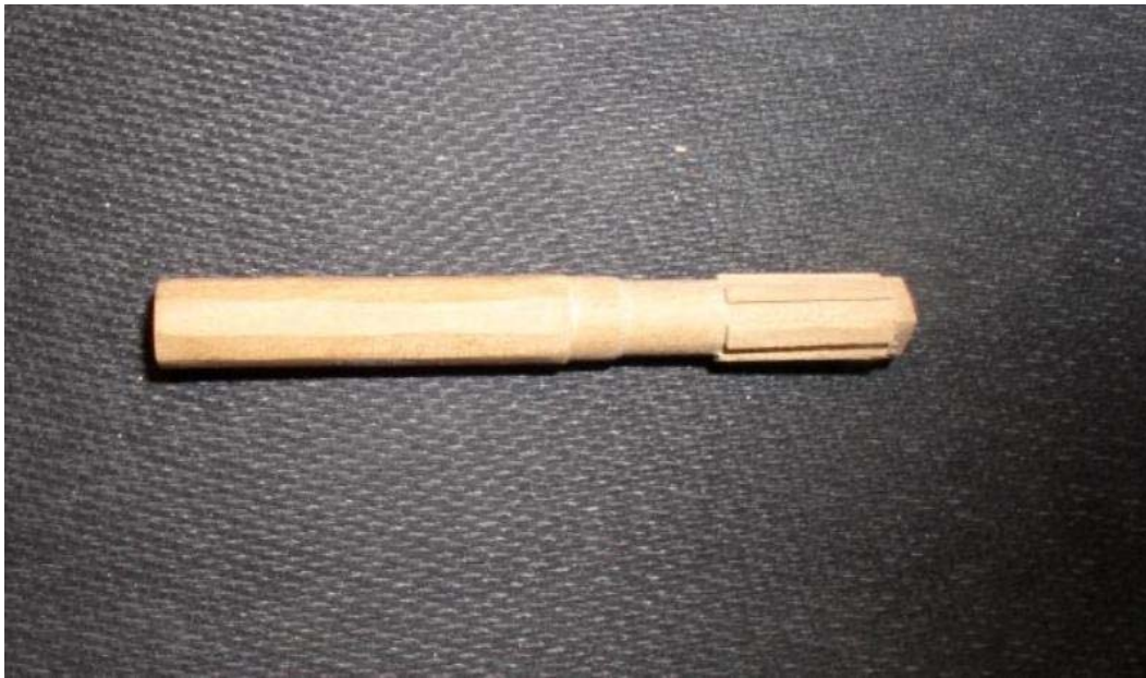
Barrel showing facets for lower whelps and facets and groves for upper whelps.
