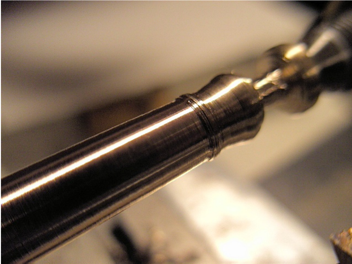
Finished muzzle and molding, all done with finishing bit.
