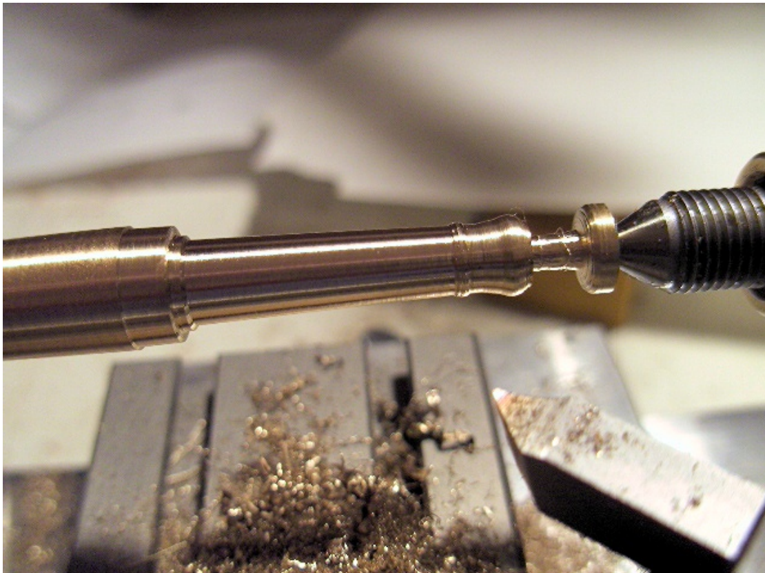
Notice the dead center and the extra material at the end of the cannon. This allows me to continue to use a dead center, which is just a little more rigid than a live one.
