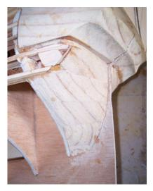
In the photo I used a Dremel with a small sanding drum to obtain the final smooth flowing shape. The final shaping needs to be done on the ship after the blocks are glued into place.
