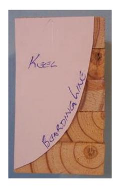
A template will need to made-up similar to the bow template from the backbone using the bearding line as the final keel shape. Place this template on the keel side of the filler blocks and mark the shape.
