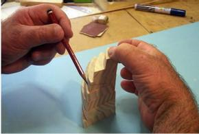
Next make up a paper card template from your plans of the keel. The bearding line will be the forward shape. This template will be placed on the backbone side of the filer blocks to establish the inside shape of the blocks.
