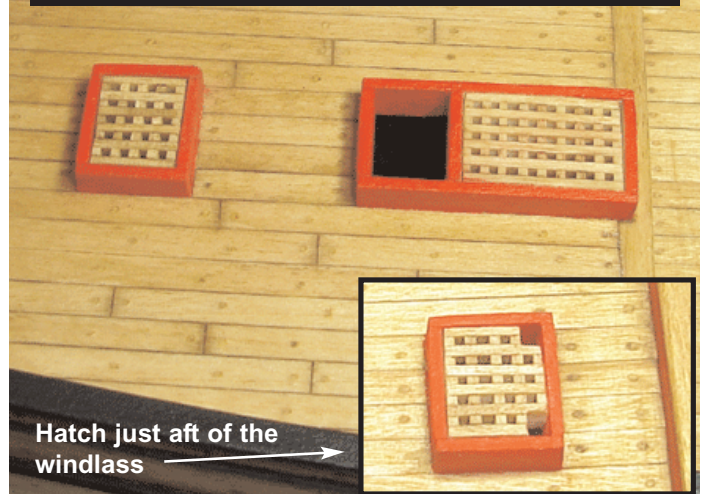
Completed hatches with gratings
