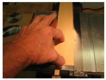
Initially I just had my fingers up on the block. Over time I've found the above hand position is more comfortable for me. I do not recommend this nor accept any liability for doing it this way, but that is what I do. Small finger is on the outside of the block and using it, in combination with my palm, is how I apply a little pressure. The above boxwood sheet is 1/8" thick and I am milling 1/32" x 1/8" strips.
