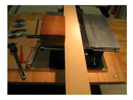
Block of wood is: 2" thick - Keeps my hand above the table and blade
