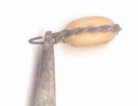
Side view of a stropped block ready for rigging to the gun tackle
