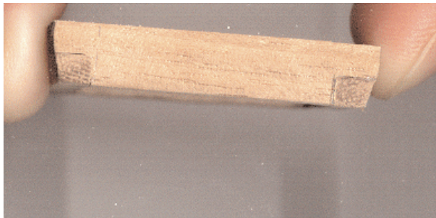
A view of the half lapped joints on the hatch coaming
