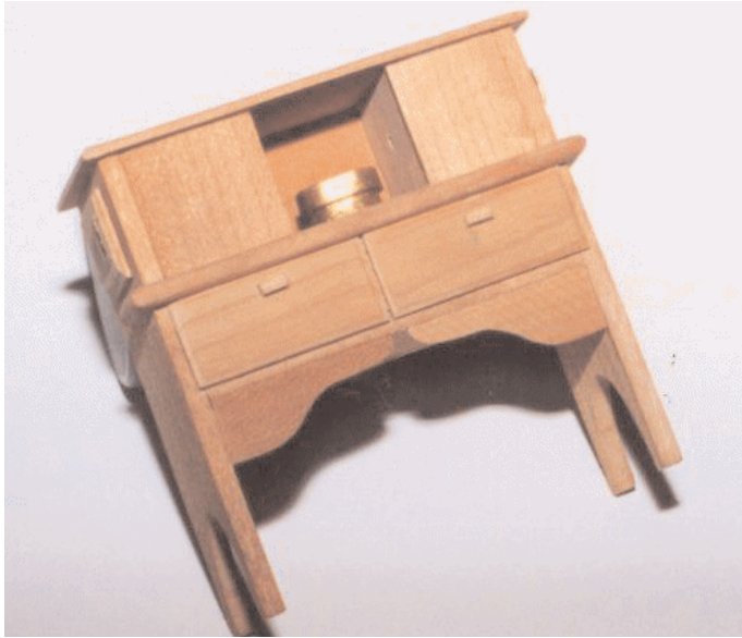
A view of another large binnacle cabinet by the author showing the compass installed
