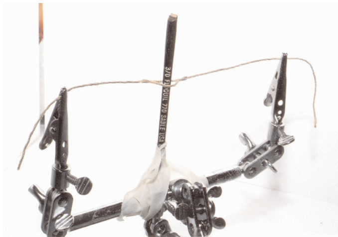
Using a modified third hand device to make a cut splice
