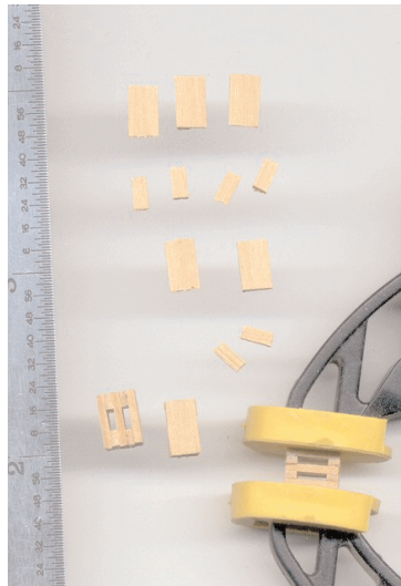
How to manufacture built up rigging blocks. Note the glued up blank and the use of bar clamps
