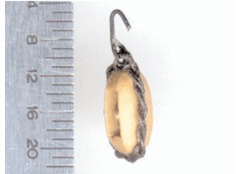
A nearly side view of the stropped block. Note the strop running right through the end of the hook
