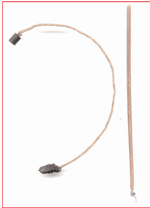
The flexible rammer and worm for the gun. Note the delicate metal on the end of the worm
