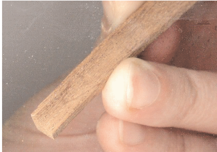
A close up view of the waterway. This was made from mahogany. A chisel was used to form the cove detail.
