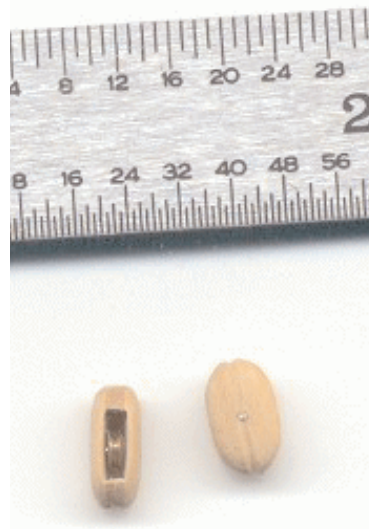
The finished blocks after shaping. Note the groove for the rope stop
