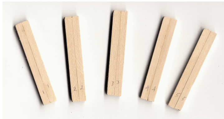
The bulwark frames for the battle station model. These have been built up of two pieces of basswood
