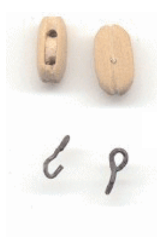
Rigging blocks with scratch build hooks
