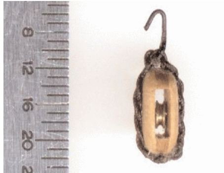
Frontal view of a stropped block ready for rigging. Note the invisible splice at the bottom of the block
