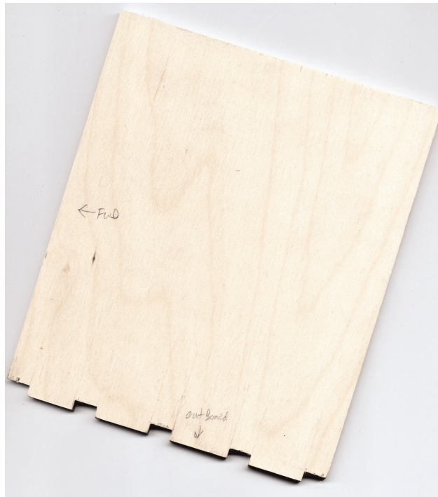
The base piece for the battle station. Note the mortises for the frames. The fore end of the base has been marked.
