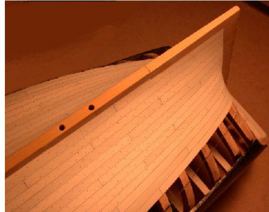
Another view at a later stage of planking. The holes in the keel are for the pedestal bolts.
